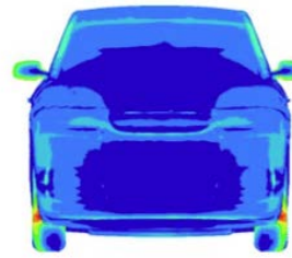
Cluster 1: Flatter windshield design with zero/one hotspot
